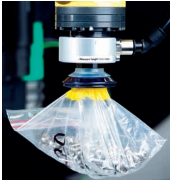
The MX suction cup has helped to deliver a smart picking concept
