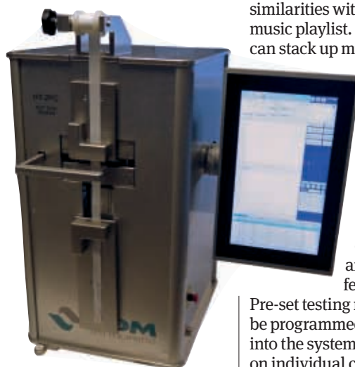
Hot tack seal strength testing is now as quick as picking a music playlist thanks to B&R software & hardware
