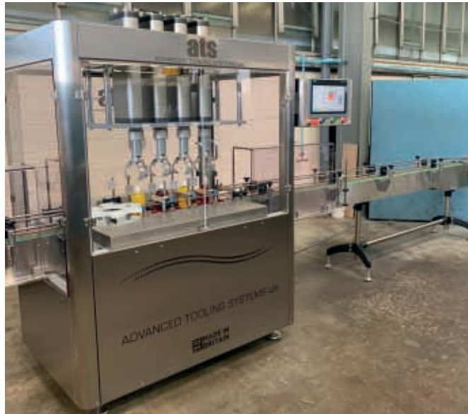
The new linear capping machine has been developed in the last five months
