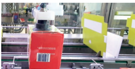
This case packer is packing cartons into SRP
