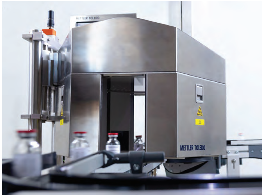
The compact systems can be integrated over existing packaging line conveyors for ease
