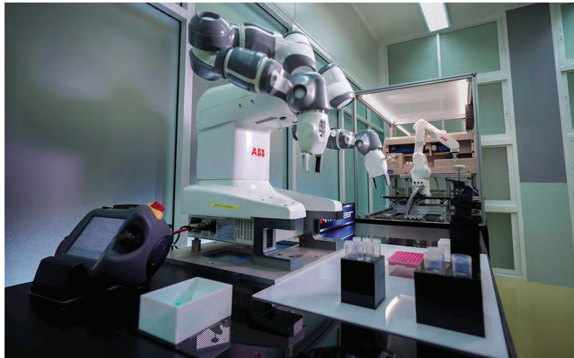
With its dual arms and versatile grippers, ABB's YuMi cobot performs a range of tasks across the pharma sector
