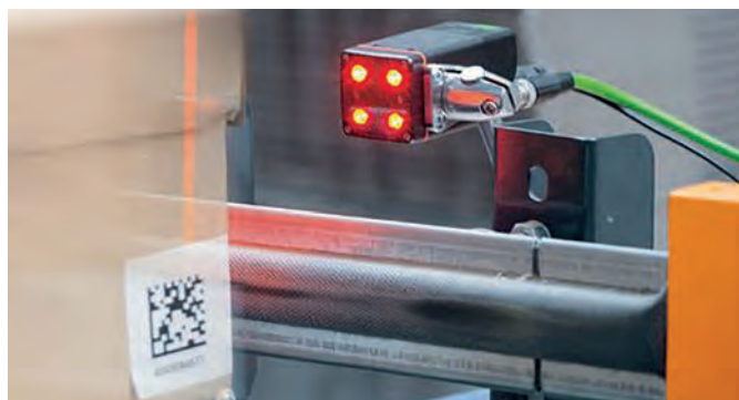
The O2I multicode reader can read almost any type of barcode or 2D code
