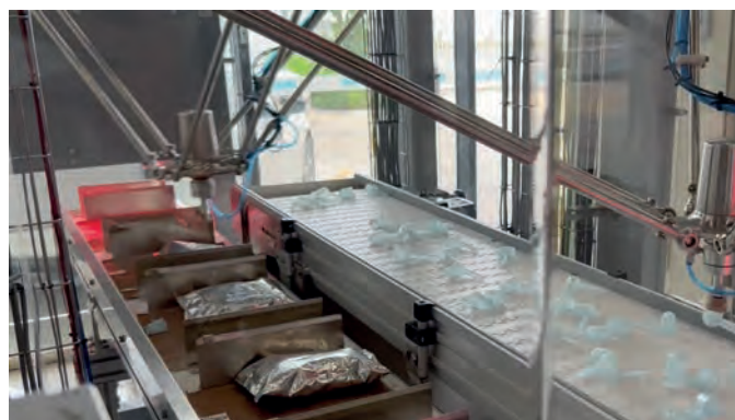
The KUKA KR DELTA robot can come into direct contact with all foodstuffs
