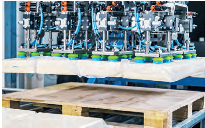
Piab's suction cups help to pick up eight blocks of cheese simultaneously
