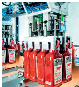
Robot loads two boxes with 8 bottles
