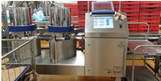
Sparc's Hera calculates ingredient weight dispensed to the exact milligram
