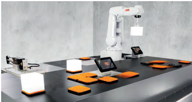
ACOPOS 6D is ideal for small-batch production with frequent changeovers
