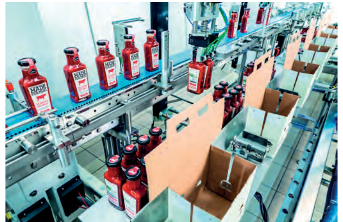
Working in counterflow, the machine handles the various bottles and cases
