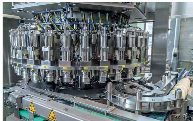
The Modulfill VFS-C can filler handles up to 15,000 containers per hour
