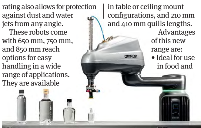
The new food-grade robots come with 650 mm, 750 mm and 850 mm reach
