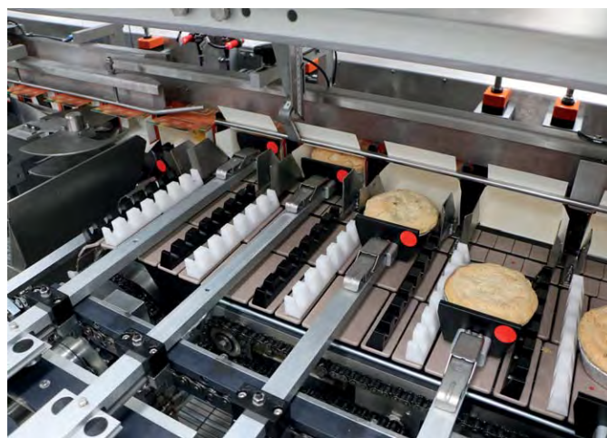
The SL903 end load cartoner offers easy, fast and repeatable size changing
