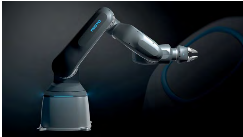
The Festo cobot's pneumatic direct drives and its light weight reduce its contact energy
