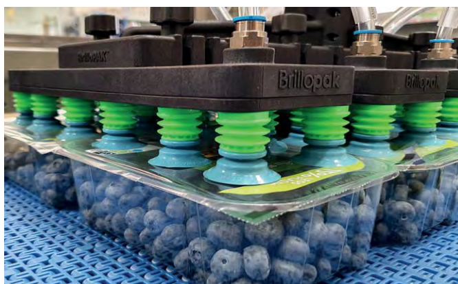
Specialist robotics with servo-driven end effectors deliver 150 punnets a minute
