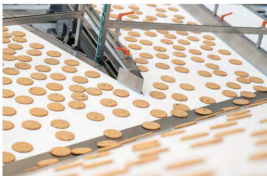
The station is equipped with belt slides to protect products
