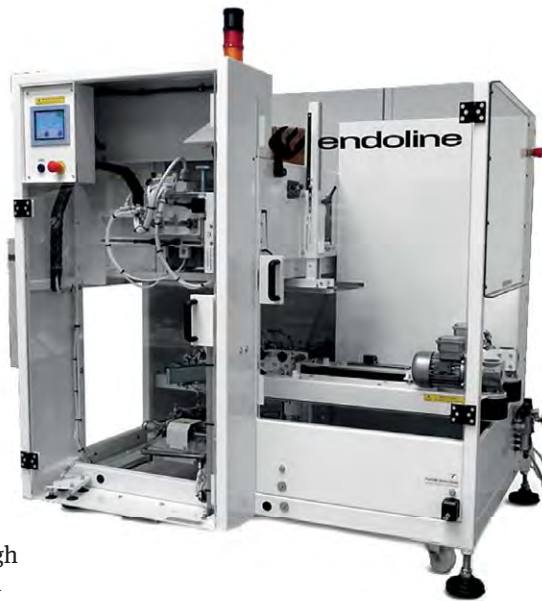
The 248 case erector now seals cases with hot melt glue rather than tapes
