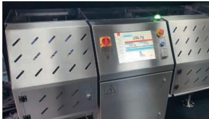
The new combination metal detector and checkweighing conveyor system
