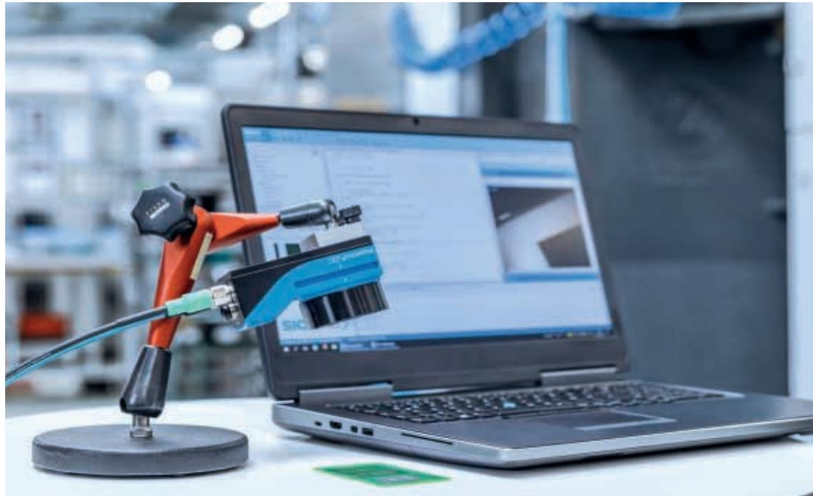
Sensor machine vision: based on image data, the camera will train for a specific task without programming knowledge
