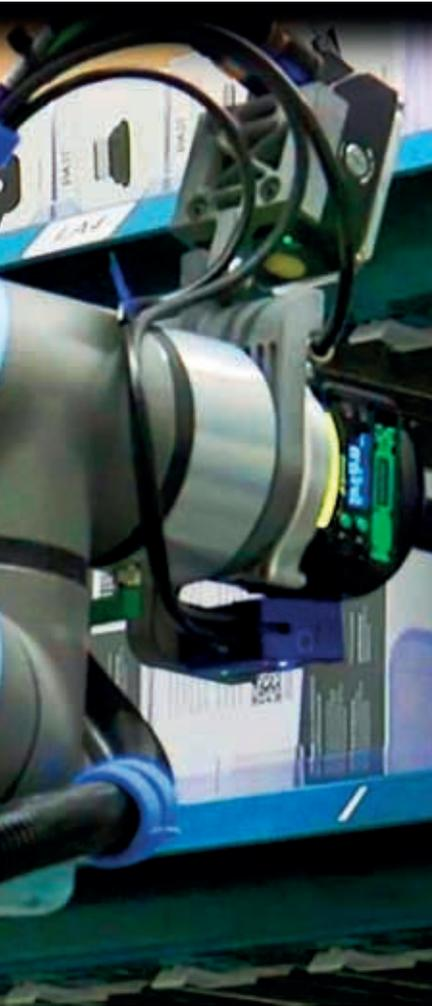
Featuring Piab's efficient COAX vacuum technology, piCOBOT comprises a vacuum pump unit and a gripper unit fitted with suction cups.
