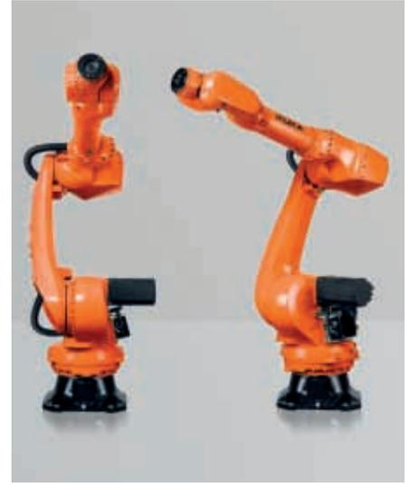
Kuka's new KR Iontec medium payload option
