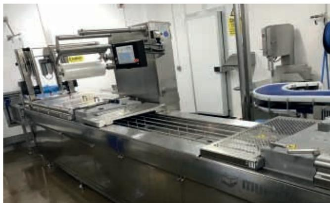
The R 215 thermoformer from Multivac in operation at JCS Fish in Grimsby
